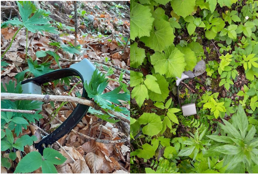
Photo 19: Two examples of retrieval of automatically opened collar on the ground after the end of monitoring period, when drop-off system enabled collar to open and be shaken off by the roe deer.
